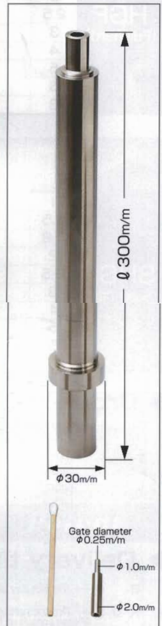
▲ Special pinpoint gate bushing
